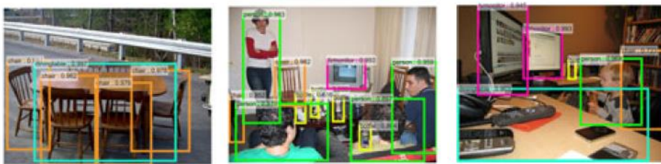
Figure 12. Chairs identified by one particularly successful DCNN, Faster R-CNN, on three Pascal VOC test images (image reproduced from Ren, He, Girshick, & Sun, 2017). Faster R-CNN speeds categorization by
